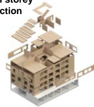
Residential multi storey modular construction
